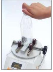
↑Opening PET bottle cap torque test
